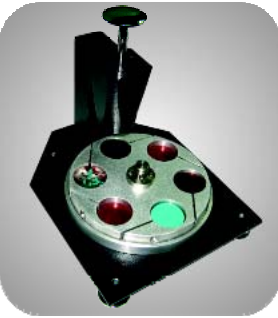
Levommat Specimen Loading Fixture to level specimens for central force specimen holders.
